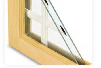
This type of divided lite window is a variant of SDL windows, except the grilles are directly integrated inside the glass panes. GBG windows keep the look of divided lite windows while having a single smooth, easy-to-clean surface. While this makes for easy maintenance, it's important to note that GBGs cannot be repainted since they are in the glass. However, they are available in a variety of colors.
